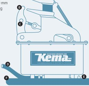
The machine is must only be used to loosen tyres. Dismantle air supply after use. Always hold onto the unit using both hands during use.
